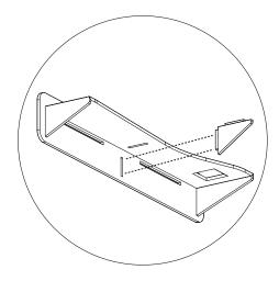
2 Insert the supporting bracket into the slot beneath the shelf
